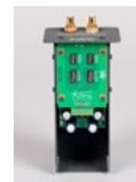
For an MC input, impedance and capacitance can be adjusted via the switches on the underside of the drawer. Two switch blocks for the right channel, two for the left. On the numbered side, the switch is open. The "ON" side is closed. Each closed switch will add the value written on the right to the other switches in the block.
